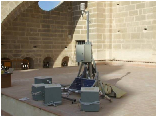
Installation of the weather station and sensors measuring surface energy fluxes (heat flow sensors) in El Salvador Church of Seville.
